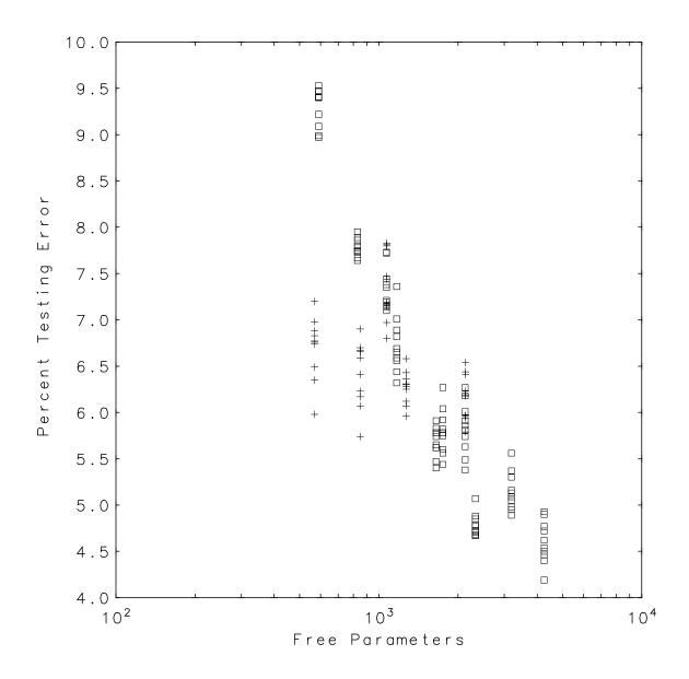
Figure 12: Testing error versus number of free parameters for MLP networks (+) and for RBF networks  $(\Box)$ .
