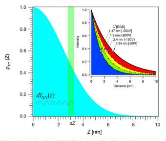
Fig. 1. Schematic of the NEXAFS depth profile of a model concentration profile of the X–Y bond. The highlighted element of thickness dz at a depth z absorbs soft X-ray of a given energy leading to an electron yield of  $dI_{XY}$ , that is subject kinetic energy loss upon traversing the distance z, characterized by the mean-free path. Inset: depth profiling as a function of entrance grid bias. The measured electron yield is controlled by the different bias, equivalently mean-free path.
