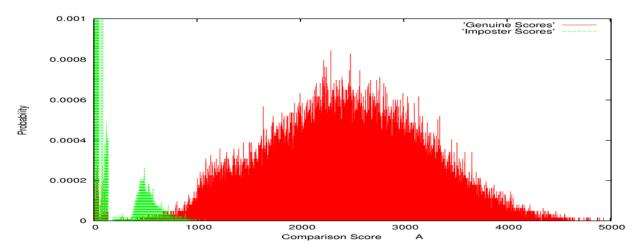
Figure 3. The discrete probability distribution functions of the genuine and impostor scores for right-index finger matching.
