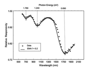
FIG. 2. Measured detector responsivity and calculated expected responsivity for purified laser-generated SWNTs. The relative expanded uncertainty of the measured values is 1.24%, as shown in three typical error bars. The level of confidence for the uncertainty is approximately 95%.
