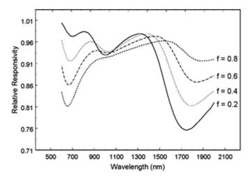
FIG. 3. Calculated values of detector responsivity depending on the fill factor of the SWNT coating, where f=1 is exclusively metallic and f=0 is semiconducting.
