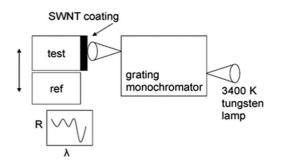
FIG. 1. Schematic diagram of the lamp and monochromator based measurement systems.
