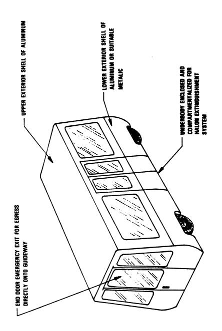
Figure 9. Vehicle exterior design features
