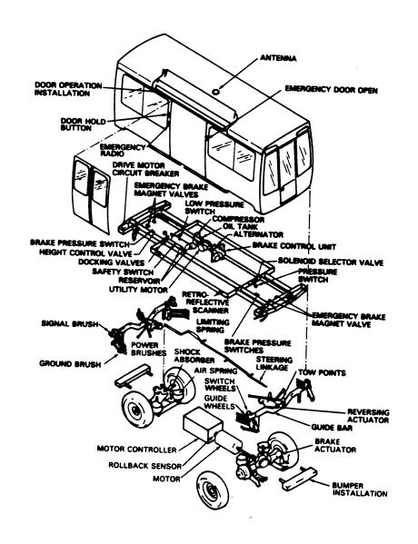
Figure 2. AIRTRANS passenger vehicle construction
