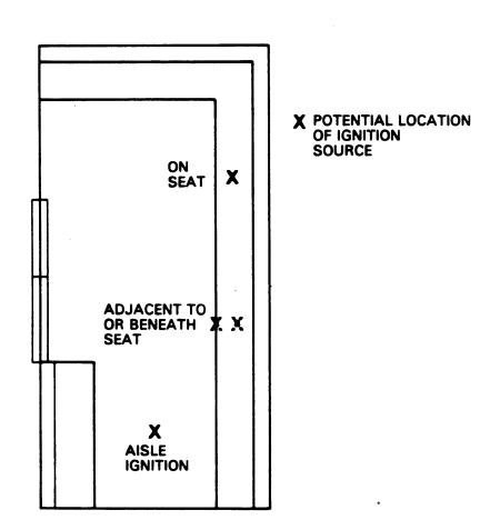
Figure 6. Probable location of ignition sources in a DPM vehicle
