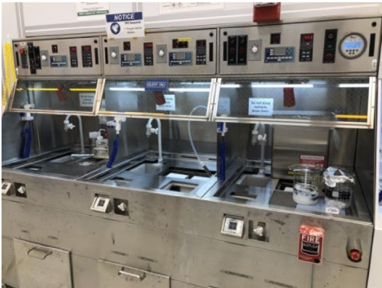
Fume hoods with adjustable sashes must be set to the proper level to protect the users face as well as to ensure adequate exhaust.
