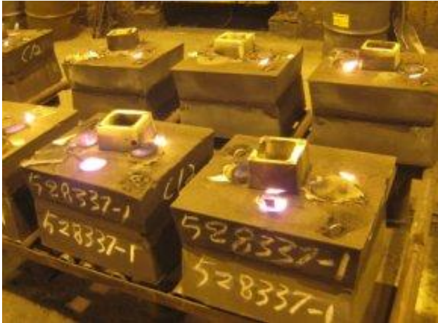
Figure 4: Filled sand casting molds.
