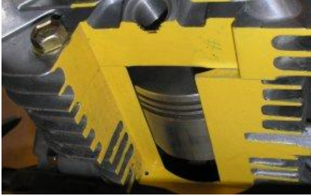
Figure 5: Cut-away view of piston and cylinder
