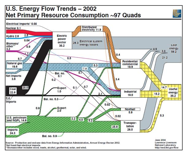
**Figure 1.** U.S. Energy Flow Chart summarizes energy streams across the national economy in terms of a common energy unit: quadrillion BTU ( $10^{15}$  BTU or  $1.055 \times 10^{18}$  joules of energy). The energy inputs are on the left, while the balance of used and wasted energy is on the right. (Kaiper)
