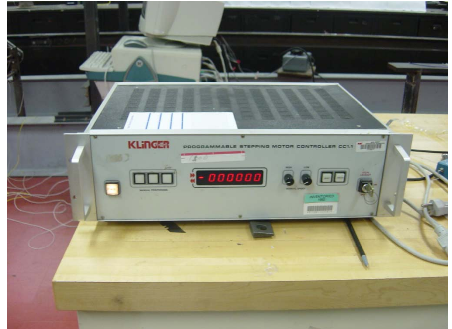
(a) Measurement set-up for strain coefficient; (b) Stepper motor driver; (b) Programmable controller (accuracy 1\mu\text{m} )
