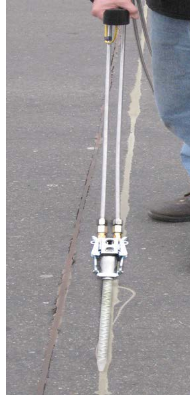
Dispensing wand with mixing head for easy deployment and cleaning
