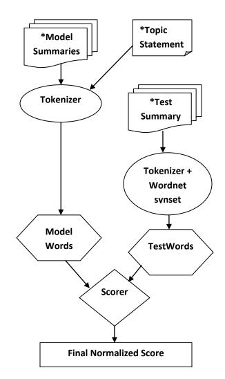
**Figure 1:** System Overview for the first run correlated with Overall Responsiveness metric. (\*  $\rightarrow$  provided by TAC)
