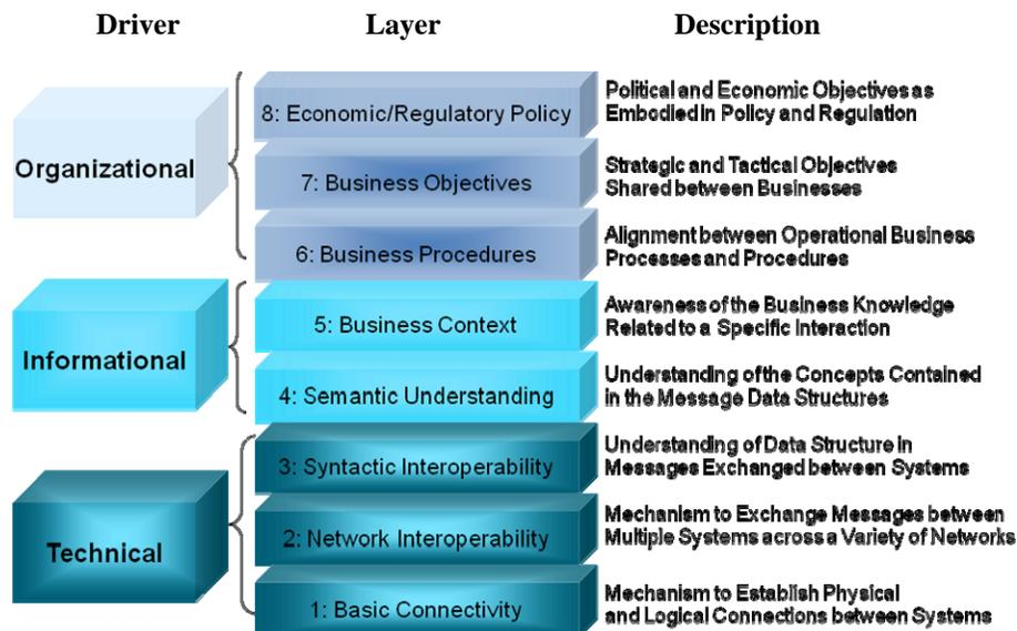
**Figure 1.** The GridWise Architecture Council’s eight-layer stack provides a context for determining Smart Grid interoperability requirements and defining exchanges of information.
