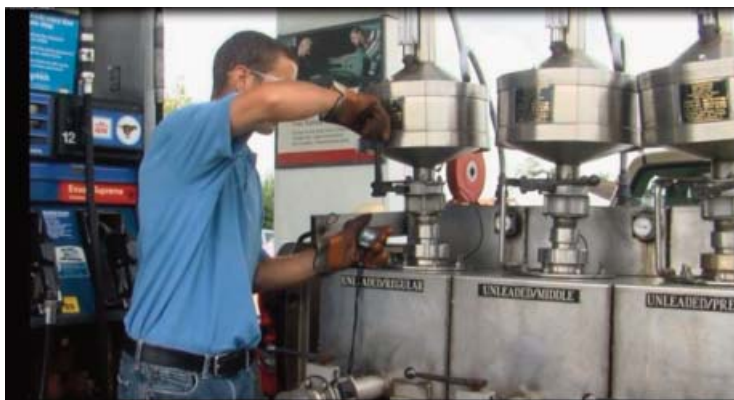
Figure 6 – Inspector Draining a Prover
