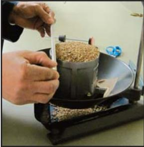
6. Hold the stoker on each end with your fingers so that the sides are in a vertical position and place it lightly on the edge of the kettle without moving the kettle (Figure 3a).
