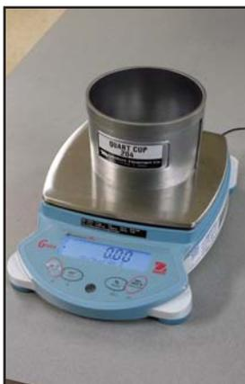
**Figure 2. Zero weight of the empty quart kettle.**
