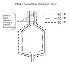
The common metals used for construction of volumetric field standards are mild steel and stainless steel. The accepted cubical coefficient of thermal expansion for the metals used to construct volumetric field standards is 0.0000186/°F for mild steel and 0.0000265/°F for stainless steel.
