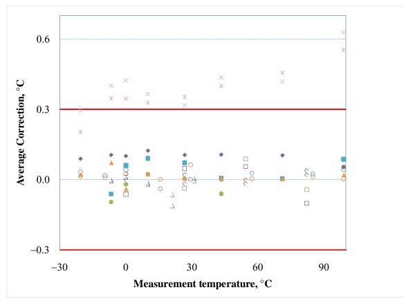
One digital thermometer model did not meet the requirement of ±0.3 °C
