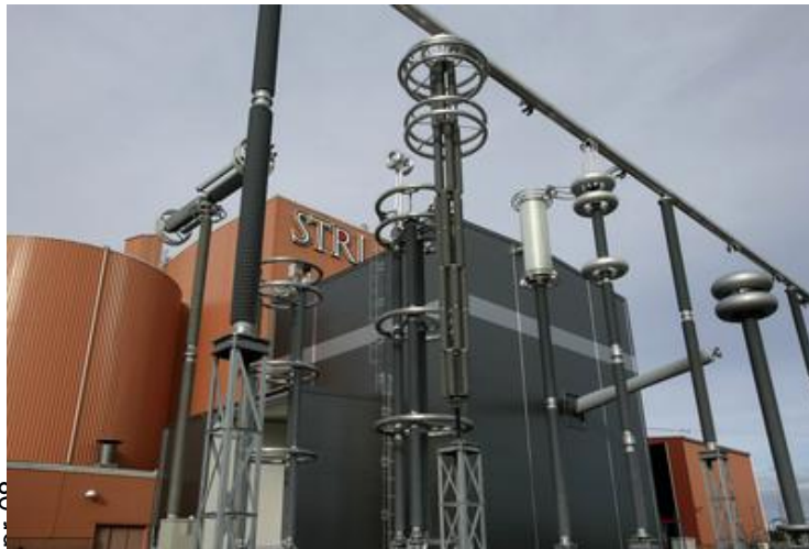
Long term test circuit for 800 kV HVDC
