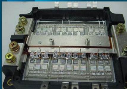
1200 V / 900 A Module Operating at 80^\circ\text{C} Heat Sink Under Stall-Zero Condition for 200 hours
