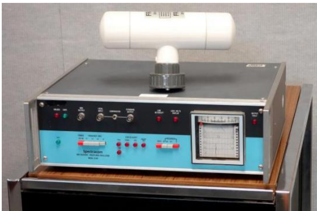
Fig. 20. Spectracom 8164 WWVB Disciplined Oscillator (A. Novick, NIST).
