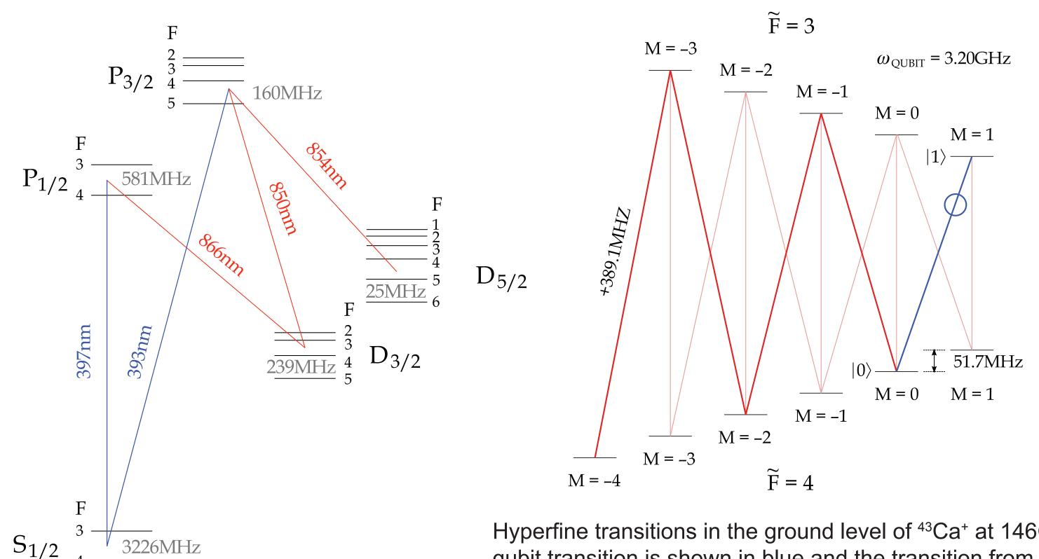
Hyperfine transitions in the ground level of <sup>43</sup>Ca<sup>+</sup> at 146G. The qubit transition is shown in blue and the transition from the stretch state to the qubit is shown in red.
