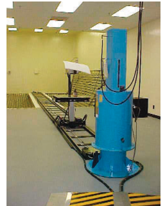
Air Force Primary Standards Laboratory calibration range for calibrating ionizing-radiation detectors.
