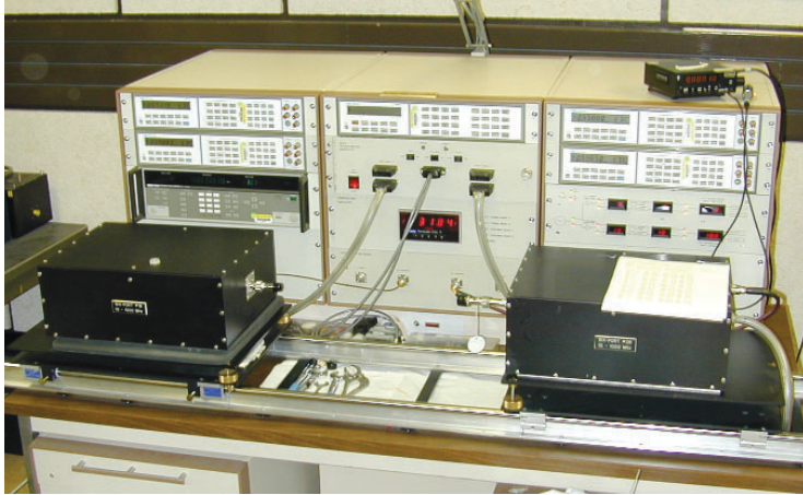
Complete six-port calibration system at NIST.
