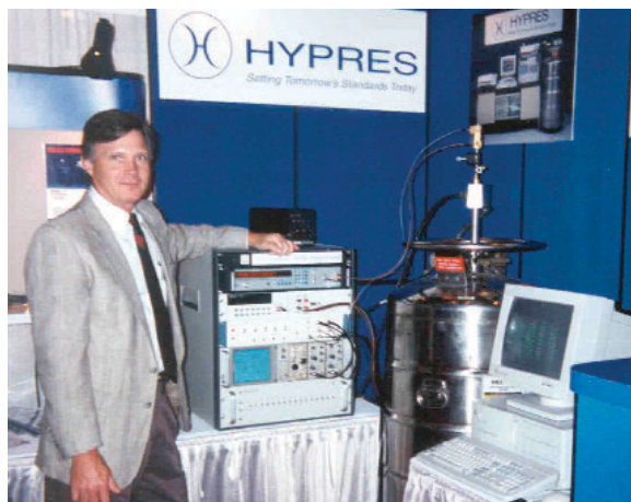
Transportable commercial Josephson junction voltage standard.
