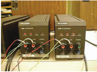
Commercial Solid-state voltage standards. (right - Courtesy Fluke Corp. left - Courtesy Datron Corp.)
