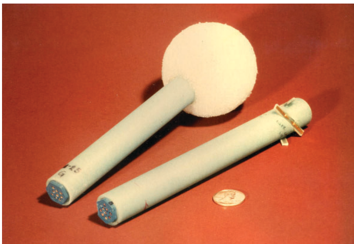
NIST three orthogonal dipole electric field intensity probe.
