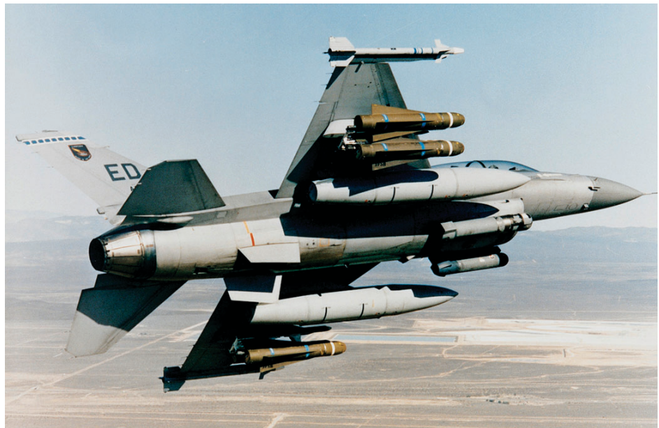
Air Force F-16 with LANTIRN laser target designator/rangefinder pod.
