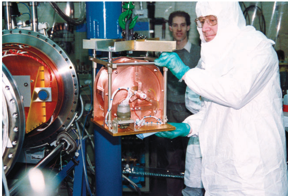
Loading the calibration fixture for the reference spheres into the LBIR at NIST.
