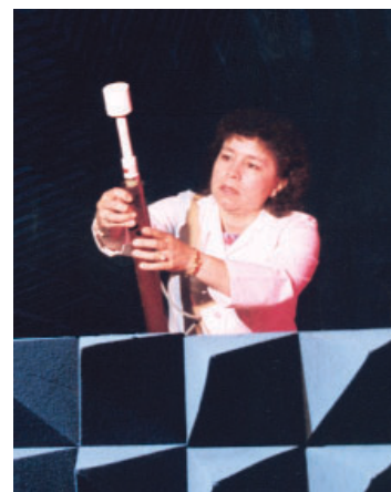
Calibrating EM hazard probe at the Navy Primary Standards Laboratory anechoic chamber facility.
