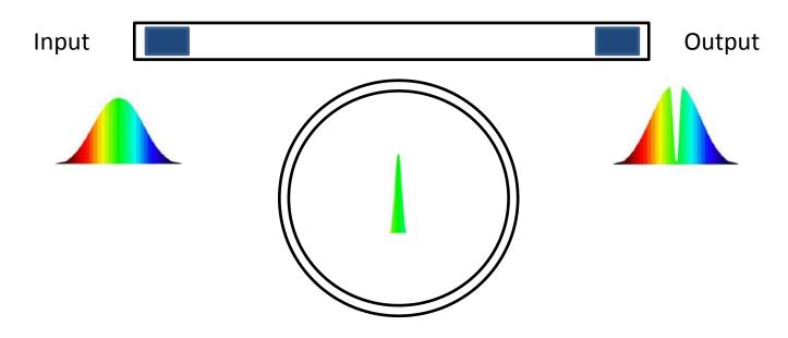
Optical ring resonators exhibit a periodic notch-filter like response where the resonant wavelength shows a temperature-dependent shift in frequency
