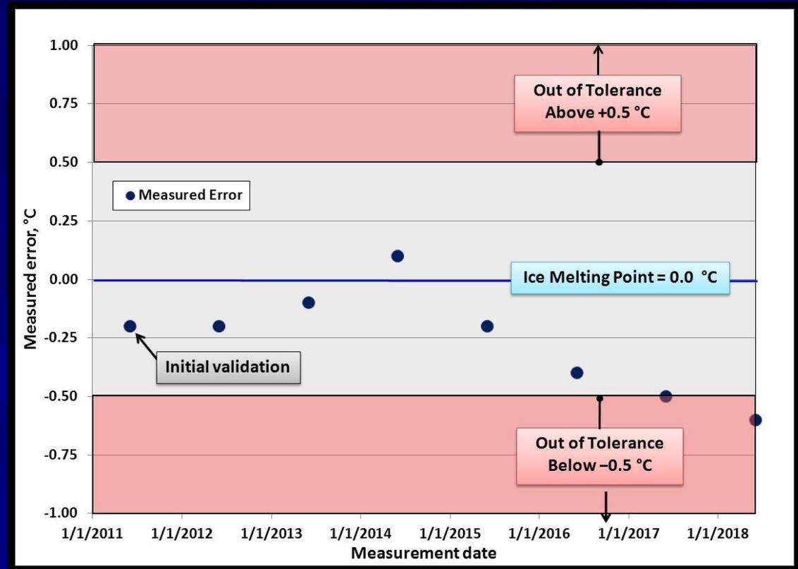
In the example control chart, we can see that a logger was validated at the ice point on an annual basis. From 2011-2017, the logger remained **in tolerance**, with a measured error  $\leq \pm 0.5$  °C
