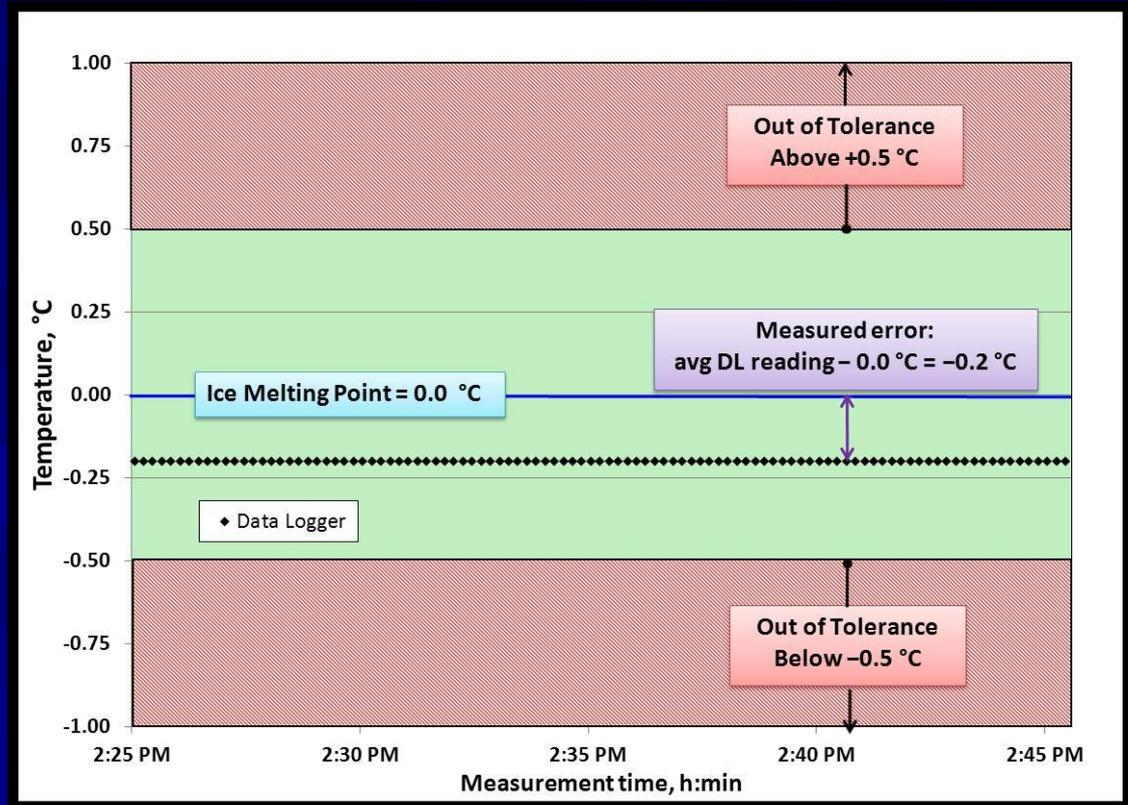
If the measured error falls within the specified accuracy ( $\pm 0.5$  °C), then the device is in tolerance and has been successfully validated at the ice melting point
