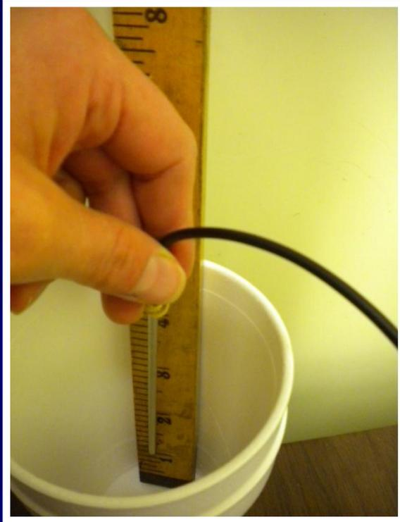
When the probe is immersed in the ice point, the probe tip should be at least 1 inch above the bottom of the cup
