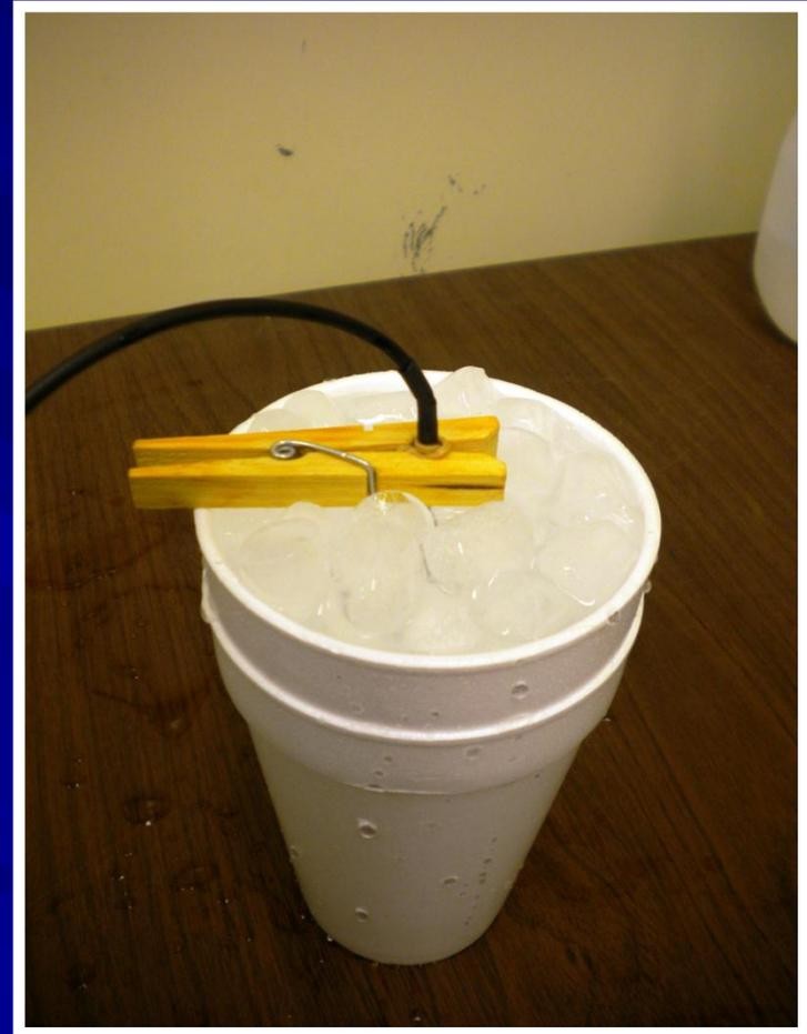
Make sure the probe is going straight down and that it is NOT tilting or touching the cup
