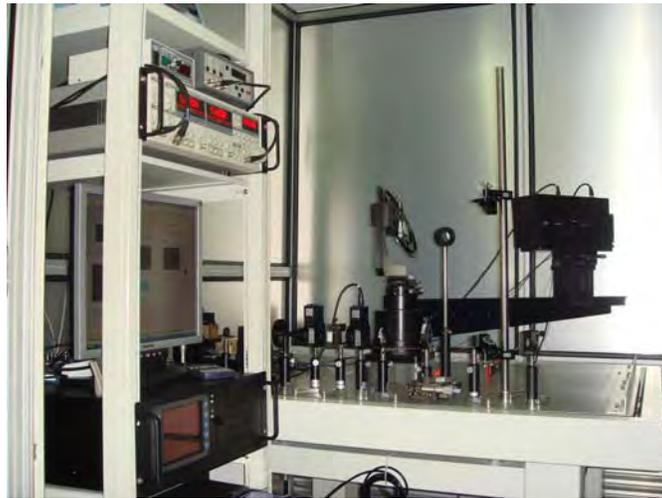
FIGURE 1. Goniometric optical scatter instrument.
