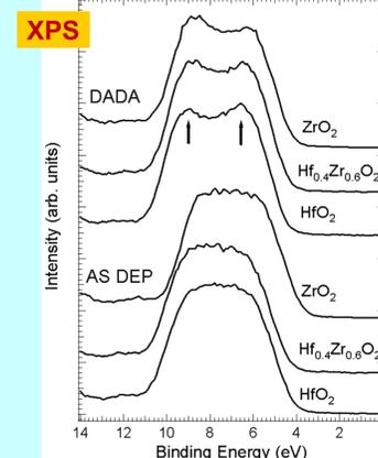
Double peak structure due to valence band splitting of O 2p bonding and non-bonding states indicates that the DADA processed films are crystalline. In the case of amorphous films one broad peak is observed.
