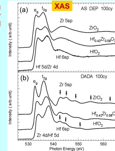
XAS at O K edge for (a) as deposited and (b) DADA processed films. Arrows show peaks in sp band and extended region. Presence of 3 peaks is signature of monoclinic phase while presence of 5 peaks is signature of tetragonal phase.
