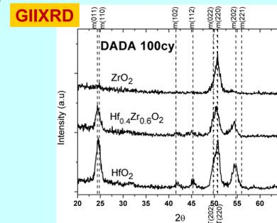
GIIXRD spectra of DADA processed films; m- $\text{HfO}_2$ ,  $\text{Hf}_{0.4}\text{Zr}_{0.6}\text{O}_2$  and t- $\text{ZrO}_2$ .
