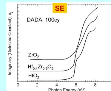
Absorption feature at 6 eV is unique to t- $\text{ZrO}_2$ . Feature is consistent with theoretically predicted self-trapped polaron in monoclinic  $\text{HfO}_2$ . [12,13]
