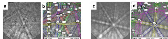
Kikuchi patterns from (a,b) 10 nm  $\text{HfO}_2$ ; and (c,d) 5 nm  $\text{HfO}_2$ . Samples were deposited by atomic layer deposition (ALD) and annealed at  $500^\circ\text{C}$  for 3 min to induce crystallinity. All patterns were indexed to the monoclinic phase of  $\text{HfO}_2$
