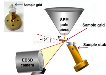
t-EBSD specimen-detector configuration. A simple custom specimen holder is used to hold a sample at  $10^\circ$  to  $20^\circ$  from horizontal.
