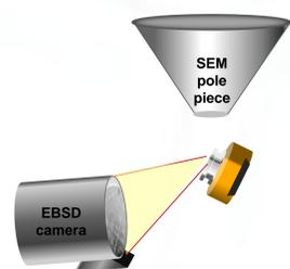
Conventional EBSD specimen-detector configuration, showing a sample tilted to  $70^\circ$  from horizontal.
