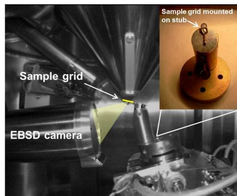
Infrared camera image of mounted sample and EBSD detector within SEM specimen chamber.
