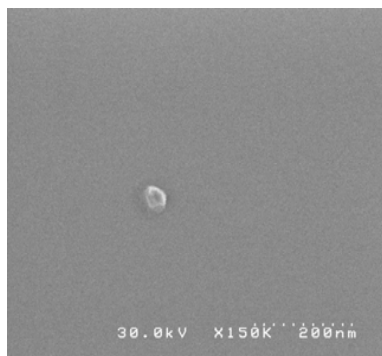
SEM picture of an Al dot (30 nm)
