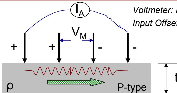
Voltmeter: Requires High  $Z_{IN}$ , low Input Offset Current
