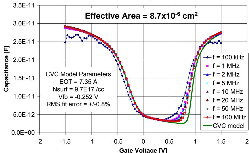
Measurement: Agilent 4294A Precision Impedance Analyzer – IV Probe mode
