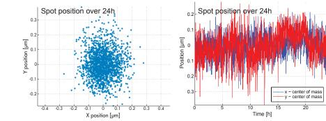
SOURCE STABILITY The spatial stability of the source is very high. The images to the left illustrate a spot centroid standard deviation of  $< 0.1 \mu m$  over 24 hours, as taken with pinhole camera mechanically coupled to the source.
