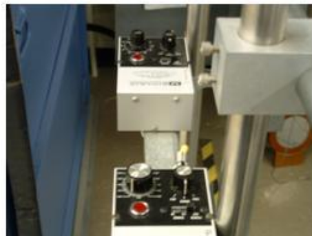
Chamber alignment controls 100 kV range
