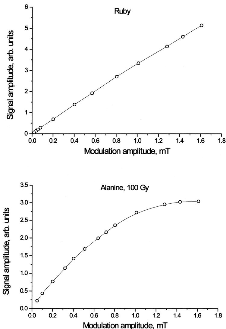
Fig. 7. Dependence of the amplitudes of ruby and alanine signals on modulation amplitude. Least-squares fit for the alanine dependence in the range 0.05–0.8 mT:  $Y = 0.474 + 3.877x - 1.252x^2 + 0.000413x/\ln x$ ; standard error of the fit is 0.012.
