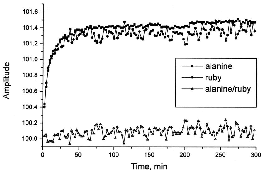
Fig. 11. Changes in the amplitudes of alanine and ruby signals, as well as in their ratio, for a dosimeter just brought in from an environment with a relative humidity higher than the humidity of the EPR laboratory.
