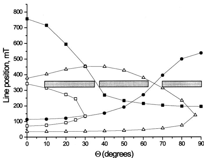
Fig. 3. Dependence of the positions of Cr(3+) lines in the X-band EPR spectrum of ruby single crystal on the angle between the crystallographic  $c$ -axis and the externally applied magnetic field. Frequency: 9.500 GHz, room temperature. Grey rectangles show crystal orientations at which the alanine signal range is free of ruby lines. (Points of different shapes correspond to transitions between different spin states; see Chang et al. (1978) for details).
