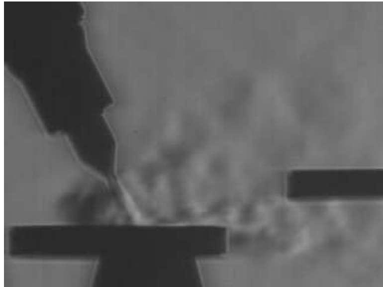
Recirculation zone formed from jet entrainment
