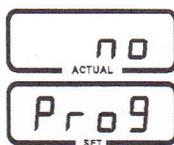
**Note:** If no key is pressed for one minute, the display always automatically reverts to Control mode.
