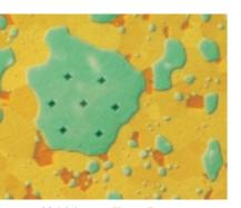
Molybdenum-silicon alloy with microhardness indentations
