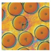
Fibre composite; interference contrast
