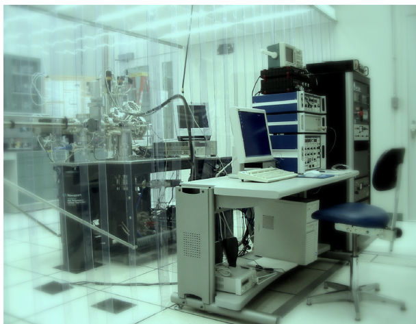
Ultra-high vacuum combined scanning tunneling microscope and atomic force microscope used for nano-scale topography and adhesion measurements.
