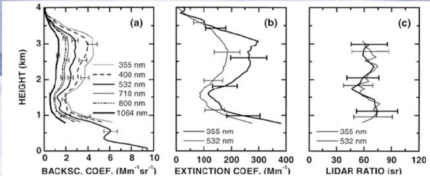
**Fig. 4.2.** Profiles of (a) backscatter and (b) extinction coefficient, and (c) lidar ratio measured on March 25, 1999 [105]. Error bars denote standard deviations caused by signal noise and systematic errors resulting from the estimates of input parameters. Because of large uncertainties introduced by the overlap effect and detector problems at 355 nm only the 532-nm backscatter profile is trustworthy down to the ground.
