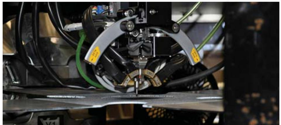
Figure 3. Close-up of x-ray stress measurement mounted on the cruciform system, positioned above a deforming sample
