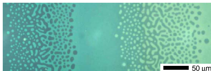
Optical micrograph showing the addition of two lamella to a block copolymer film as the film thickness changes from 81 nm (left) to 117 nm (right).
