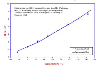
Thin film expansion data are needed to model the mechanical integrity of multilevel microelectronic chips that are subjected to temperature and humility changes.
