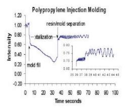
The sensor can be used to detect asymmetric shrinkage when the two sides of a product shrink at different rates. Such asymmetric shrinkage can be an indicator of warpage in the molded product. The simplicity of design that uses inexpensive components enhances the probability that R&D laboratories and processors will use the sensor to monitor molding operations.
