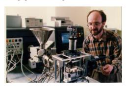
instrument that permits visualization of polymer blends during extrusion. Many plastics sold today are combinations of two or more incompatible polymers. Mixing these components to obtain the proper morphology is key to producing materials with desired properties. The instrument consists of a stroboscopic microscope and laser-based light scattering system that performs real time non-invasive microstructural measurements in multi-phase polymeric materials during polymer processing.
