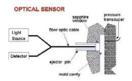
The sensor is a simple and inexpensive device consisting of a diode laser light source, optical fibers for light transmission, a sapphire window interfaced with the mold cavity, and a silicon diode photodetector. As light is transmitted into the mold, it reflects from any interface at which there is a change in the index of refraction, such as the interface between resin and sapphire window and the
