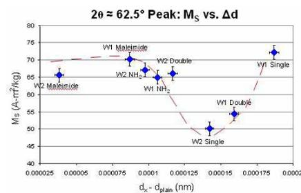
Saturation magnetization data vs. change in lattice constant.
