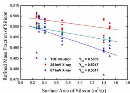
Refined diffraction data for SRM 676a
