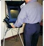
**ACTIVATE THE MACHINE** by inserting the Activation Card into the yellow slot on the lower left-hand side of the machine.
