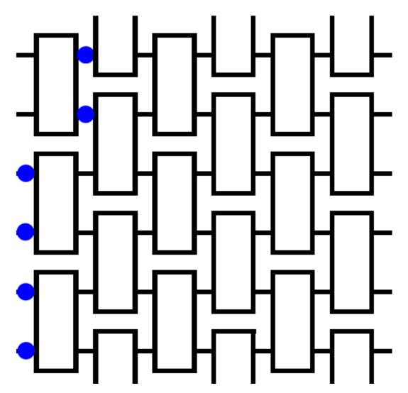
Definition valid time-configuration t (informally): for no pair of qubits interacting at time t in the circuit is the clock of one qubit past t and the clock of the other qubit before t.  $H_{circuit}$  preserves the subspace of valid time-configurations
