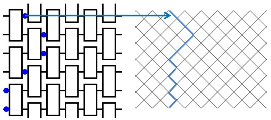
Picture on the right: each gate is represented as square and blue string is vertex in the graph. Points in time are on the edges. Strings (vertices) are connected by transitions  $\langle \leftrightarrow \rangle$ .
