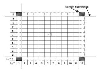
**Fig. 6.** Enlargement of the central region of Figure 5. Link-cell periodic boundaries become processor domain boundaries. Dashed lines correspond to ghost cells.
