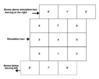
**Fig. 8.** A nine processor 2-D domain decomposition and neighboring layers resulting from application of an applied strain consistent with the Lees-Edwards boundary condition.
