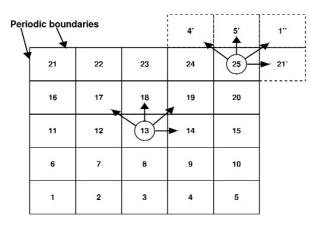
Fig. 2. Schematic 2-D representation of the link-cell algorithm.
