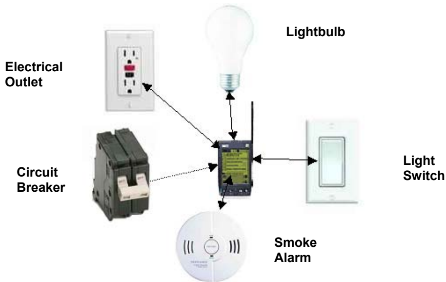
Figure 2.4.1 Example variety of objects networked using IEEE802.15.4 (from [22]).
