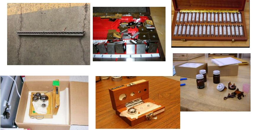
Most cases are designed to protect the gages in the lab, not for shipping. On the left, the box has allowed a high stakes billiards game with precision gages. Wires, on the other hand, are in separate tubes.
