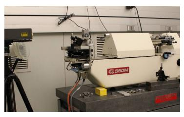
If the scale is positioned parallel to the machine motion and centered on the contacts the effects of pitch and yaw errors in the machine motion are considerably reduced.
