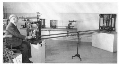
Plate 34: Albert Bonhoure operating the Ruprecht No.1 balance in Room 5 of the Observatoire, date unknown but probably in the 1940s or 1950s; all balances were operated at a distance to avoid heating by close proximity of the operator. (*Courtesy BIPM*.)
