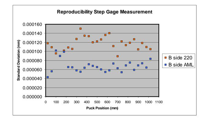
This shows the history of our 1020 KOBA run on the same machine, the Moore M48. The top data is the old  $\pm 0.1$  °C laboratory. The bottom data is from the AML with its  $\pm 0.01$  °C laboratory. The difference is dramatic, lowering our uncertainty by 50%.
