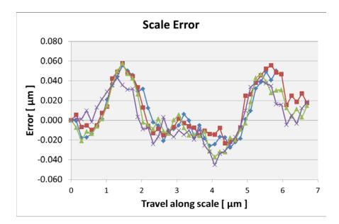
The graph on the left shows a typical response, it if from a Heidenhain Brochure, and it is about 1% of the pitch. On the right is the error measured on a measuring machine in my lab. Our machine has 4  $\mu$ m pitch so the error should be about 40nm, and it is.
