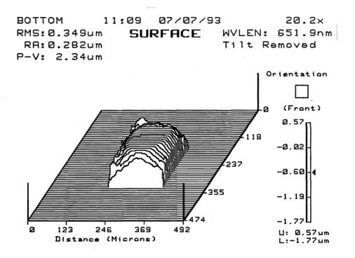
We also assume we know the geometry of the contact. This is the surface of one diamond contact on our gage block comparator. It is remarkably flat with a diameter of over 100  $\mu$ m, reducing the deformation by 30 nm. This is larger than our uncertainty!
