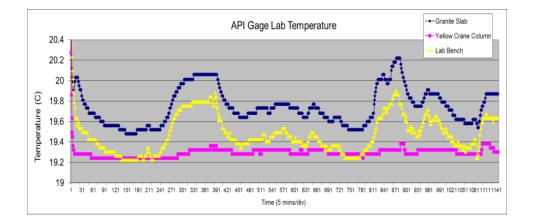
In our conventional labs, where the temperature is controlled to about 0.5 °C we see temperature differences of about that size. Large machines have a large thermal mass, effectively filtering the temperature changes..
