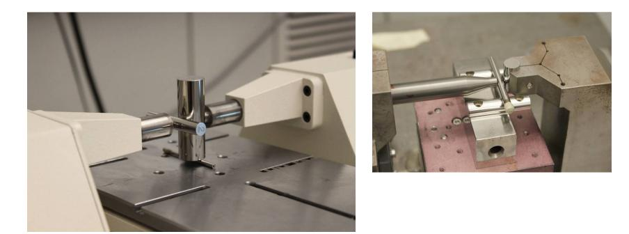
For small cylinders supported by two parallel half-rounds, the micrometer force will align the gage surface to the micrometer contact. As the cylinders get bigger, static friction becomes greater and alignment errors are common.
