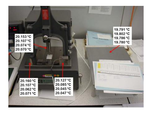
Here we have the aluminum soaking tray next to the comparator. While only separated by a few inches the temperature differs from the comparator by 0.3 °C.
