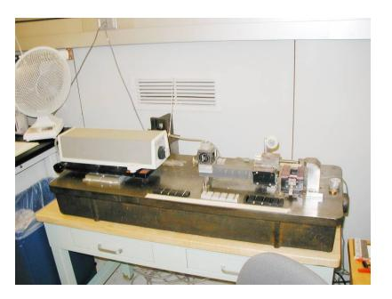
This is our holder for balls and wires. The "V" grooves have cone do not provide as much thermal conduction as gage blocks on a plate, but these are generally small gages with little thermal mass.
