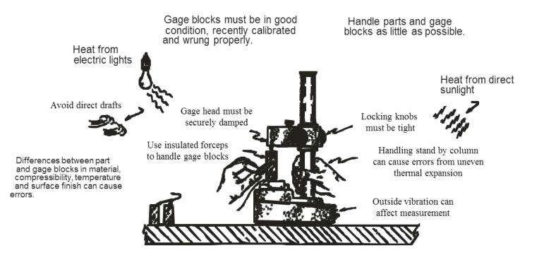
Figure 11-37. All sources of potential errors should be consciously investigated whenever a high precision measurement is made.
