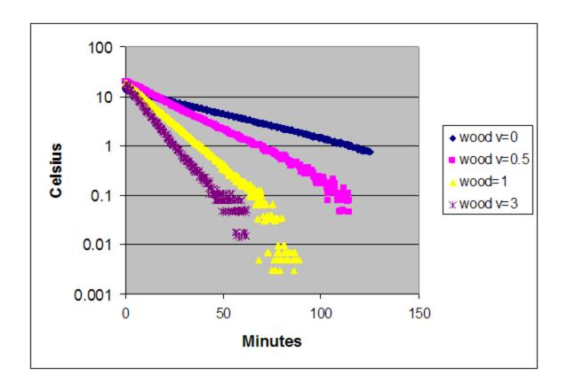
This logarithmic plot shows that the exponential decal model works very well, and the addition of the fan has a dramatic effect.
