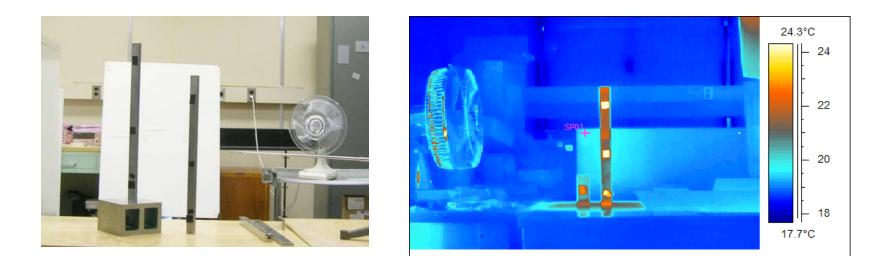
Each of the 500 mm gage blocks have three strips of tape as the thermometry target. The fan can be seen in the background and the anemometer extends horizontally from the right side of the picture.
