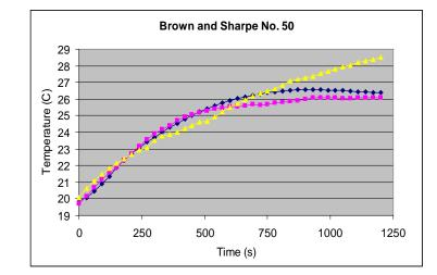
Using a thermal expansion coefficient of 12 PPM/°C and the fact that the maximum range of the Brown and Sharpe #50 micrometer is two inches, the error in measurement caused by a shift of 6 °C is  $3.07 \ \mu$ m. The same test with a micrometer with a thermal insulating plate reduced the effect considerably.
