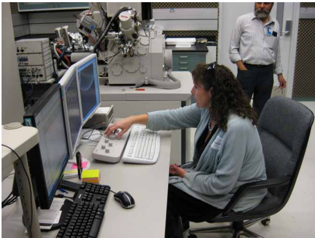
Lisa Wheelock catches on quickly and moves the sample around to investigate interesting sections of the cricket. The cricket was coated with \sim 10 nm of gold to make it conductive so that it will show up when the beam of electrons hits it.
