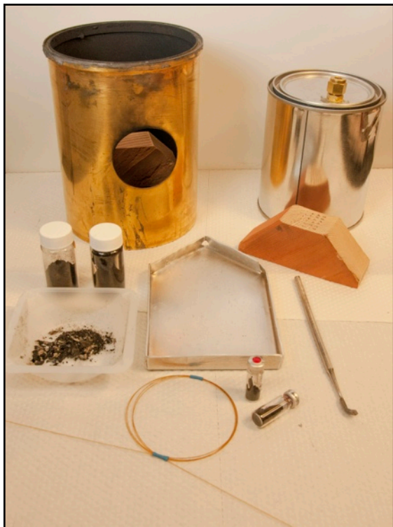
Shown here are the tools for testing arson samples using NIST's new PLOT capillary method. Credit: NIST
