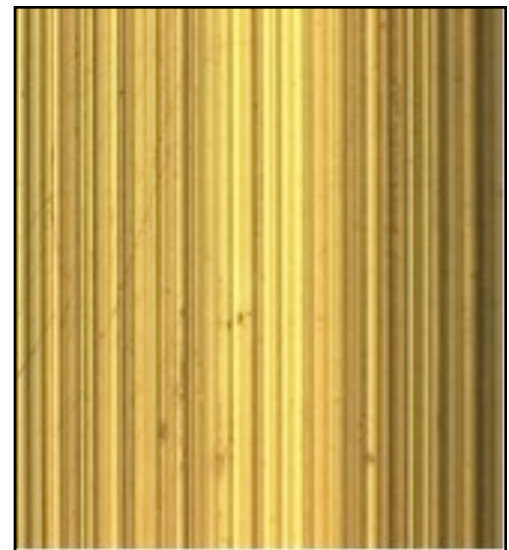
The land impression on NIST SRM 2460 Standard Bullet
