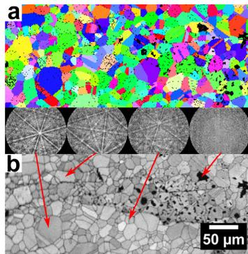
The EBSD software also produces a map of a parameter called "pattern quality" (above, bottom) which is an assessment of the contrast in the diffraction pattern. Areas where the sample has undergone severe plastic deformation will tend have low pattern quality.
