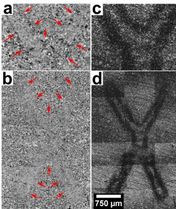
The imprint is faintly visible in the forward scattered image and very clearly visible in the EBSD pattern quality map. Low **pattern quality** in areas with sub-surface damage reveal the image of the stamped letter X.
