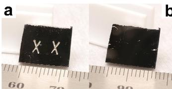
The imprint was then polished away, beginning with 120 grit SiC paper down to 0.05  $\mu\text{m}$  colloidal silica, and finishing with electropolishing in a solution of 50%  $\text{H}_3\text{PO}_4$  and 50%  $\text{H}_2\text{SO}_4$
