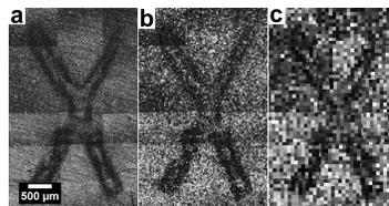
The original EBSD scan (above left) required 9 hours for a single letter due to a (software limited) maximum pixel size of 6.72  $\mu\text{m}$ . Undersampling the collected data by 5x (above center, 33.6  $\mu\text{m}$  pixels) and 10x (above right, 67.2  $\mu\text{m}$  pixels) still shows unambiguous reconstruction of the stamped letter.
