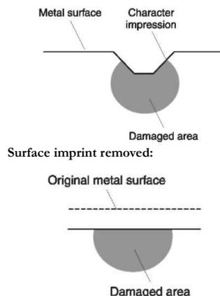
A number of techniques (acid etching, heat treating, etc.) can partially or fully restore serial numbers. However, many of these methods can produce unsatisfactory and/or ambiguous results.
