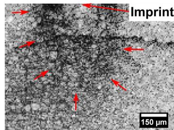
The image quality map of the cross section (above) shows that the deformation is detected via EBSD pattern quality mapping to a depth of about 520  $\mu\text{m}$  beneath the bottom of the imprint. **A criminal would therefore have to remove about 760  $\mu\text{m}$  of material (140  $\mu\text{m}$  imprint, 520  $\mu\text{m}$  sub-surface damage) to render a serial number undetectable by EBSD.**
