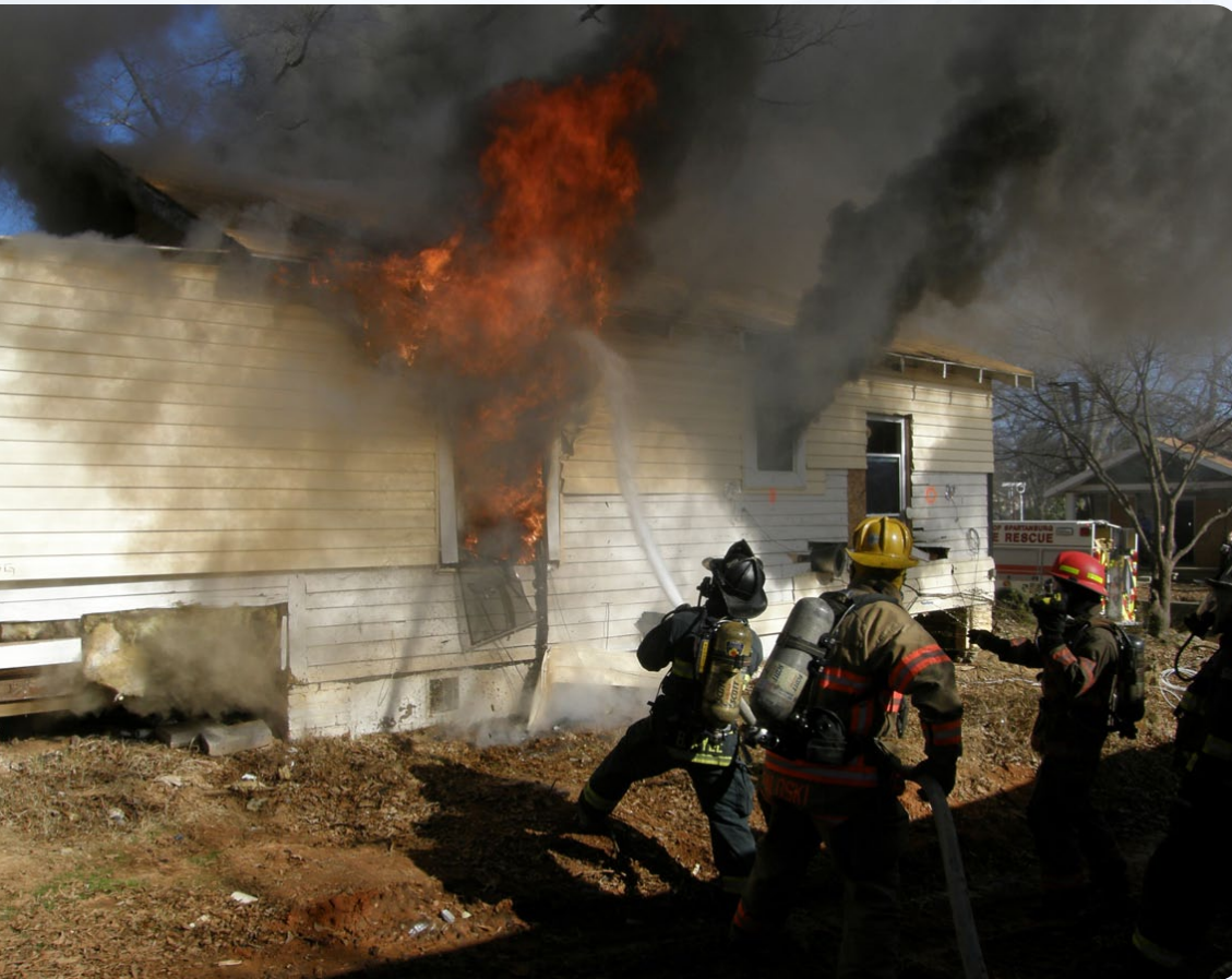
Firefighters in Spartanburg, S.C., battle a 'test burn' of an abandoned house in an experiment to demonstrate new techniques for combating flashover, an extremely dangerous phenomenon in fires. Researchers from NIST, the International Society of Fire Service Instructors, and state and local fire and safety officials participated in the tests the week of Jan. 20, 2013 Credit: Madrzykowski/NIST
